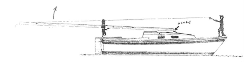
The mast should be approximately plumb to the waterline and should not lean over the bow or over the stern. The forestay and backstay should be carried quite snug. The tension between the upper and lower side stays, or shrouds, should be adjusted so the mast is straight athwartships when sailing in a good breeze. In general, the shrouds should always be keptrather taut, but they do not have to be exceptionally tight.
