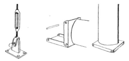
6. Position the mast so that it may be raised from aft to forward with the butt of the mast in the hinged mast step.
